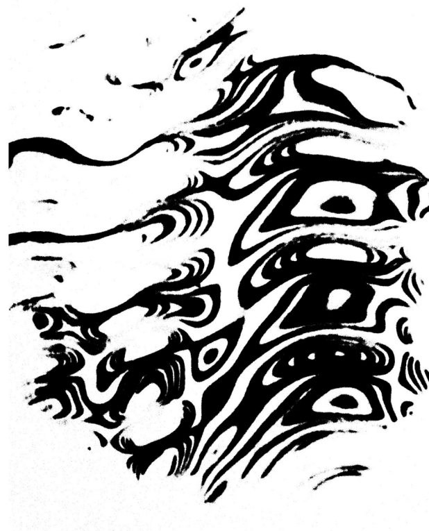
Schlieren picture of a falling liquid film
